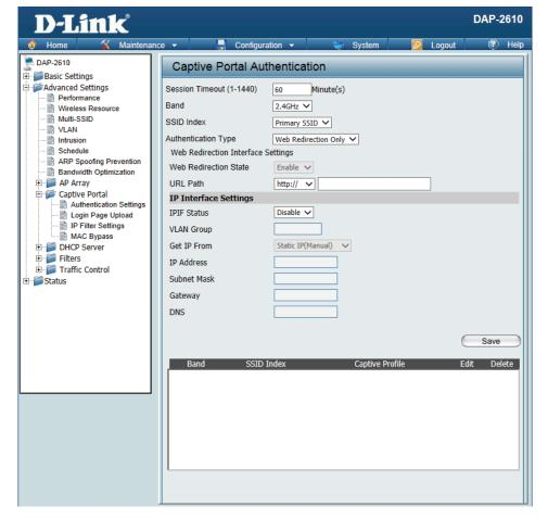
**IP Address:** Assign a static IP address that is within the IP address range of your network.
