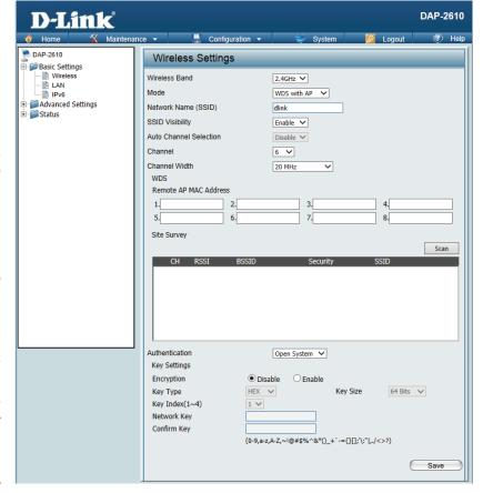
Remote AP MAC Address: Enter the MAC addresses of the APs on your network that will serve as bridges to wirelessly connect multiple networks.
